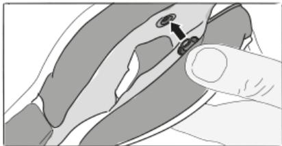
HOW TO REMOVE THE INNER LINING?
